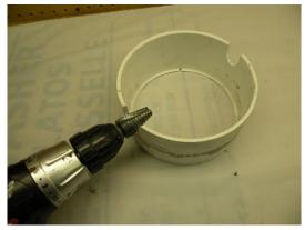
Cut the 6-inch PVC pipe coupling in half along the circumference. This should create two pieces as shown above. The height of the piece will be 3 inches which is normally too high for your lantern to sit inside of without the sides hitting. Use a progressive drill bit to notch out the two sides so the lanterns bottom sites firmly at the same level as the bottom of the PVC piece. Set the lantern in place and test for stability. This piece will become the cradle on the bottom of the carrier.
