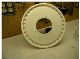
Take the 4-inch vent and center in on the lid. Trace a line around the vent. Cut out the center circle with a fine blade in the jigsaw.
