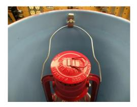
Set the lantern in the cradle and let the handle rest against the side of the bucket. Depending on the type of handle clip you use, mark and drill a hole to mount the clip with the  $\frac{1}{2}$  x 20 bolt and wing nut.
